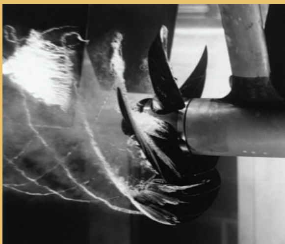
Figures 1.8. Cavitating propeller model in a water tunnel experiment.
