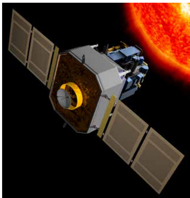
Artistic rendition of the SOHO spacecraft in space. The telescope is facing the sun; the panels acquire energy from the sun; the small dish antenna at the rear sends data gathered back to Earth.
